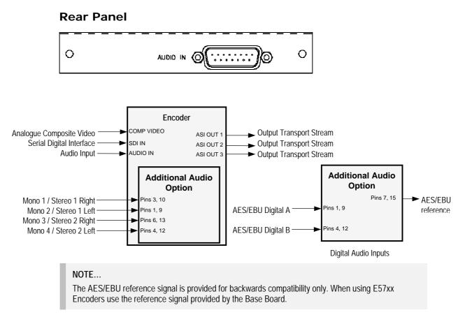
Figure 3.1: Additional Audio and Linear PCM Option (M2/EOM2/AUDLIN)
